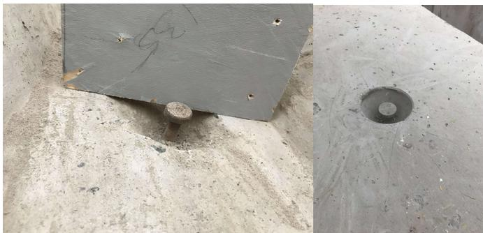
Figure A left hand image with anchor showing clear evidence of creep strain due to repeated use. Right hand image showing anchor set below concrete surface in newly manufactured concrete.
